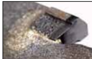
The MicroGeo diamond teeth eliminates the large space between teeth.
